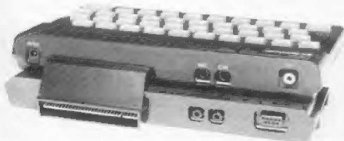
The Interface 1, which attaches to the Spectrum at the rear edge connector. It fits under the Spectrum, tilting the computer forward by 20 degrees
